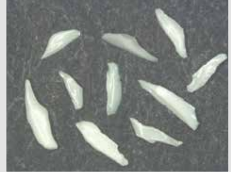
Macrostructure of individual Extra Sharp exploded CERPASS DGE®-0789 grains.
