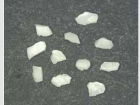
Macrostructure of 36-grit Strong Blocky-shaped CERPASS XTL®-0560 grains.
