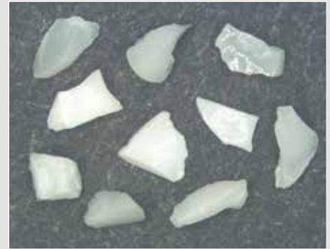
Macrostructure of 36-grit Weak Splintery-shaped CERPASS XTL®-0565 grains.
