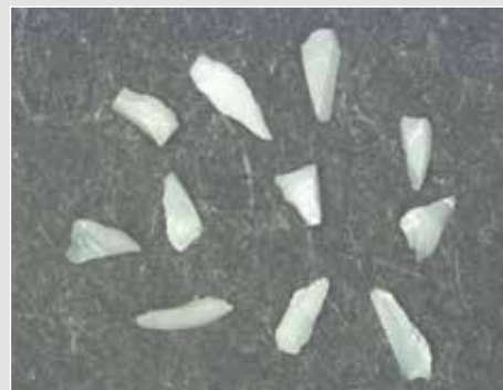
Macrostructure of individual Weak Splintery-shaped CERPASS XTL®-0570 grains.
